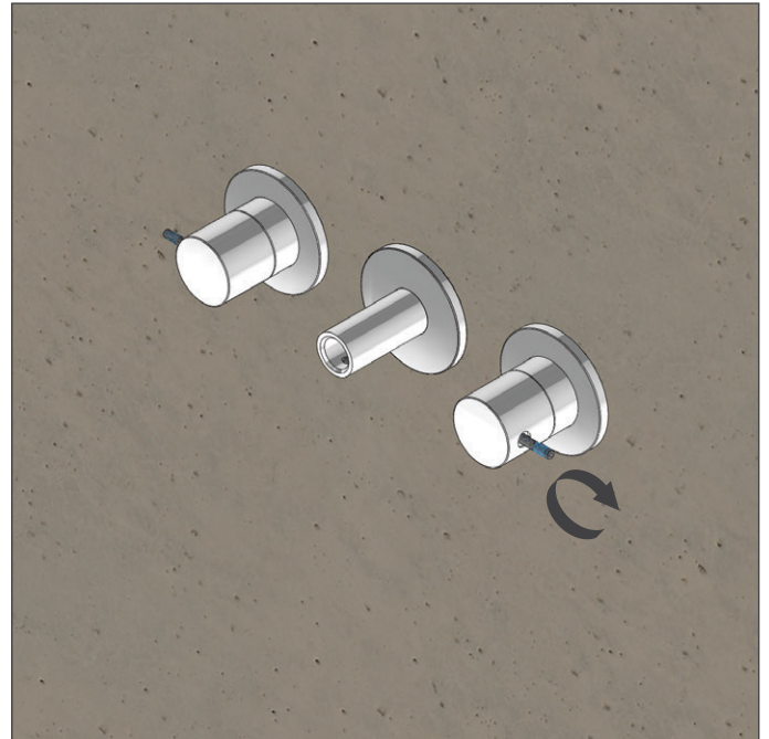
Tighten long hex screw to secure handle
