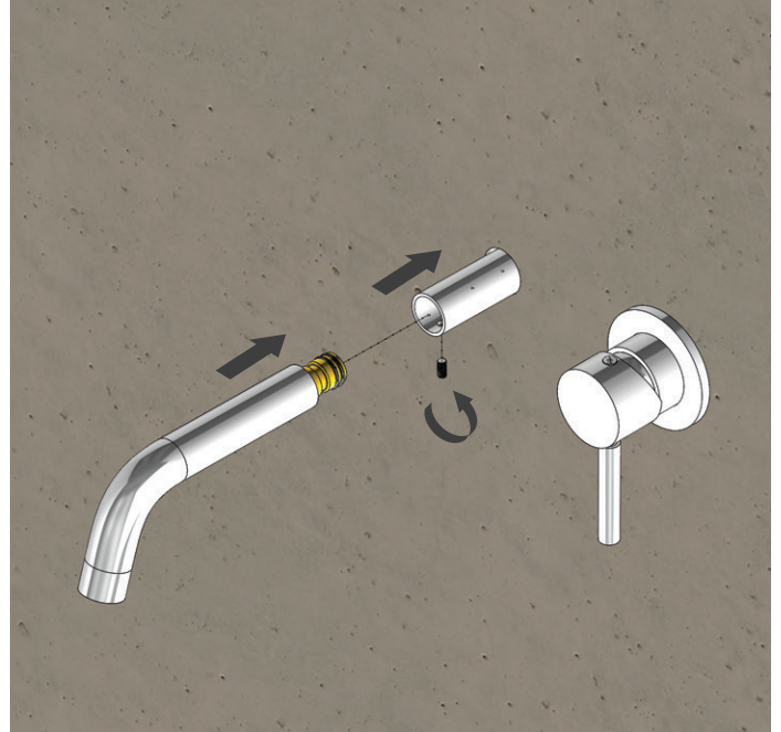
Insert spout back piece by twisting. Then insert spout front piece and tighten hex screw.
