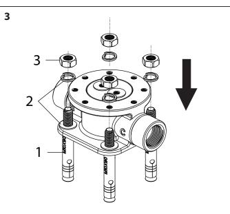
Mark holes for floor bolt installation. Install valve using bolts (1). Secure head bolts with washers (2) and nuts (3). Ensure valve is perfectly level.
