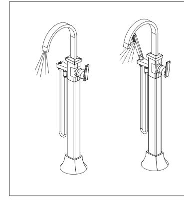
After Installationis complete remove the aerator with the provided aerator key and flush the water lines. Turn on the hot and cold supply lines and allow water to flow for approximately 1 minute. After flushing re-insert the aerator.
