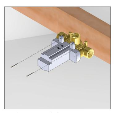
Fix Valve on wooden plank
