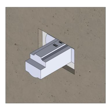
Install Drywall and Tile. Ensure finished tile surface is between the min and max marks on the mud guards.
