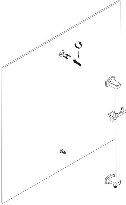
Bring out supplied 1/2" connection and install top slide on connector with supplied screws
