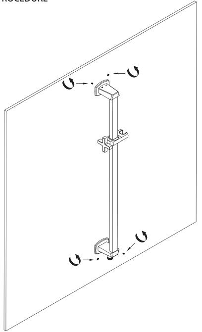
Tighten hex screws to secure slide bar to wall
